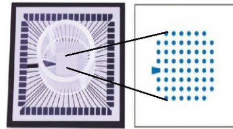
**Fig. 1** A picture of MEA used in these experiments (<https://www.multichannelsystems.com/>) (left panel) and magnified depiction of electrode arrangement (right panel)
